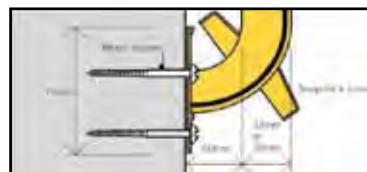
Fixing to timber
