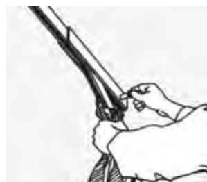
2. Place cassette into the bridge at angle locating against post inside bridge
