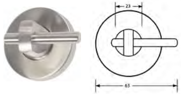
Offset Pin & Thumbturn Supplied with GRI 711 indicator, latch and keep LH/RH universal mount
